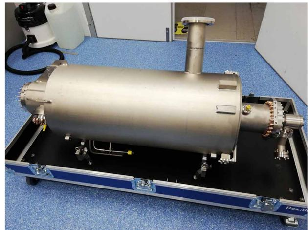
Figure 1: ESS high-beta 704 MHz cavity.
