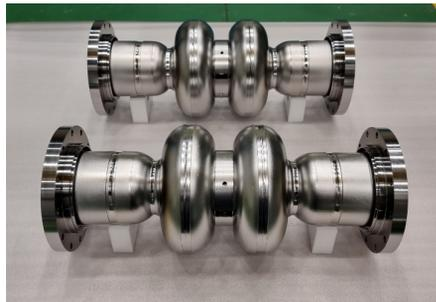
Figure 1: Fabricated niobium double-cell cavities.
