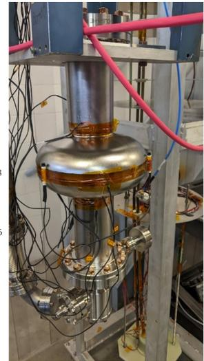
Figure 1: Illustration of the test setup. Left-hand diagram shows the positions of the thermometers (C) and magnetometers (F). Right-hand photo shows the instrumented cavity on the test insert.
