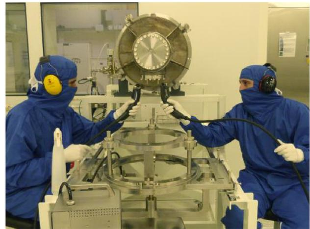
Figure 1: Manual cleaning operation on coupler to cavity assembly workstation.
