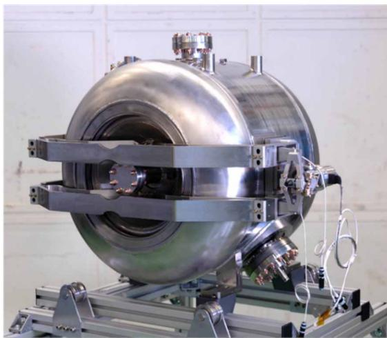
Figure 1: Prototype SSR2 cavity equipped with its tuner.
