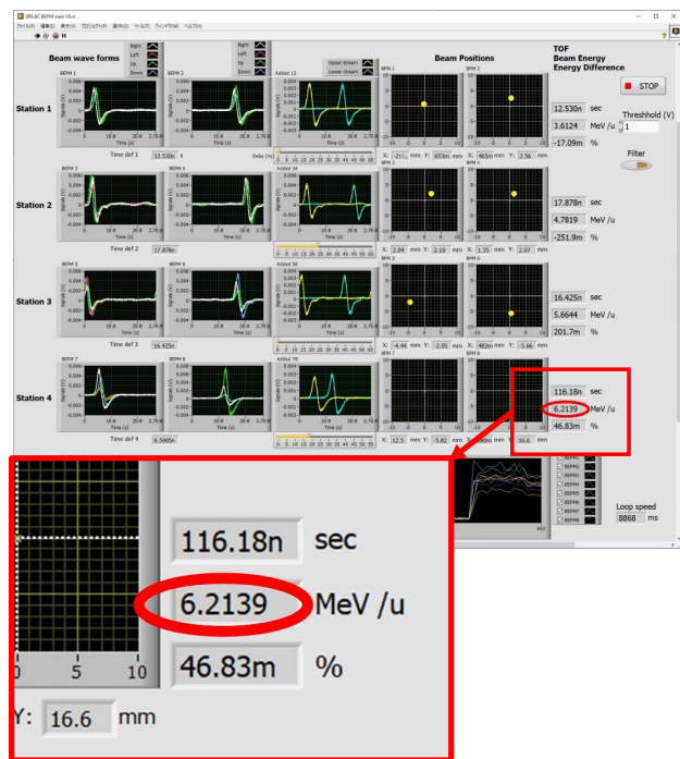
Figure 15: Measurement screen of the BEPM system (preliminary version). The specified energy of 6.2 MeV/u was obtained.
