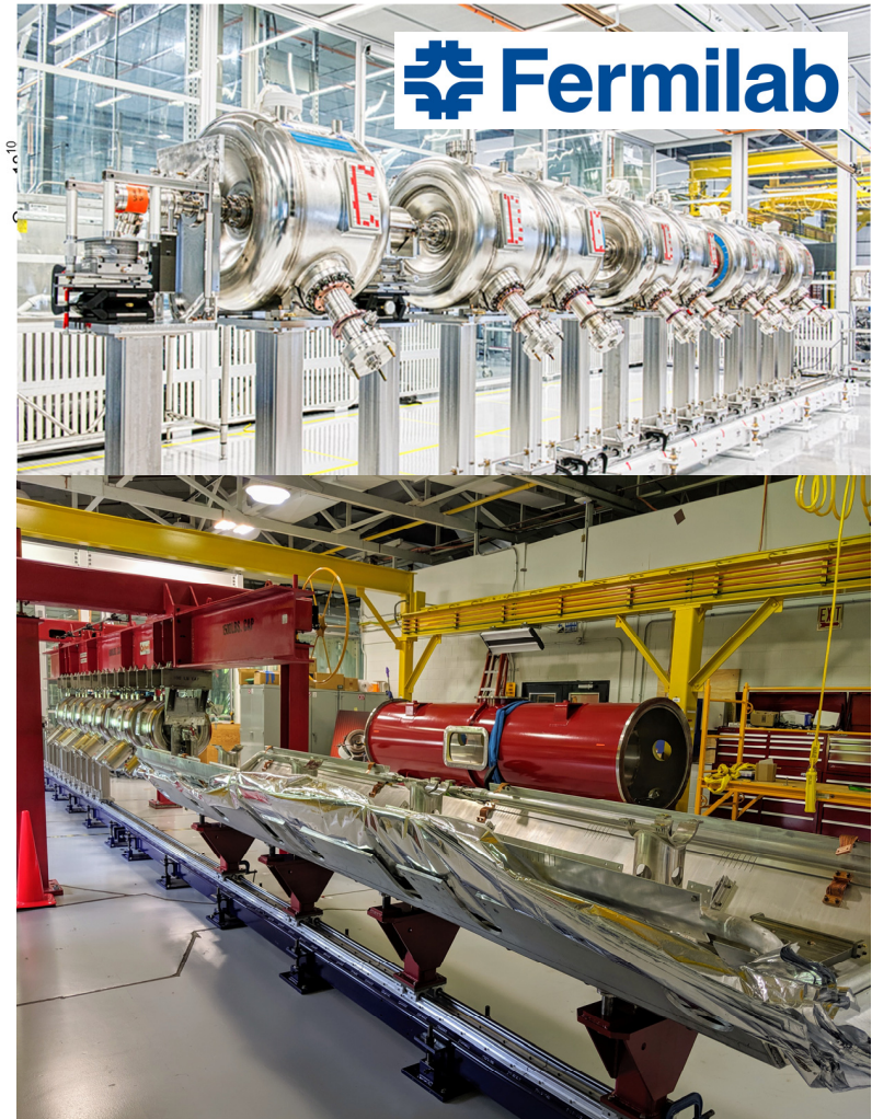
SSR1 cryomodule cold mass assembly
