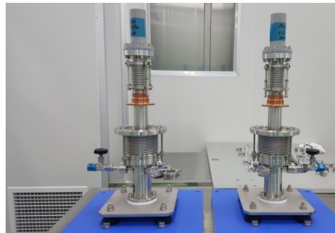
QWR Coupler for RAON (IBS/RISP) 81.25MHz
