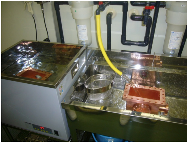
Ultra-pure water rinsing with ultra-sonic agitation
