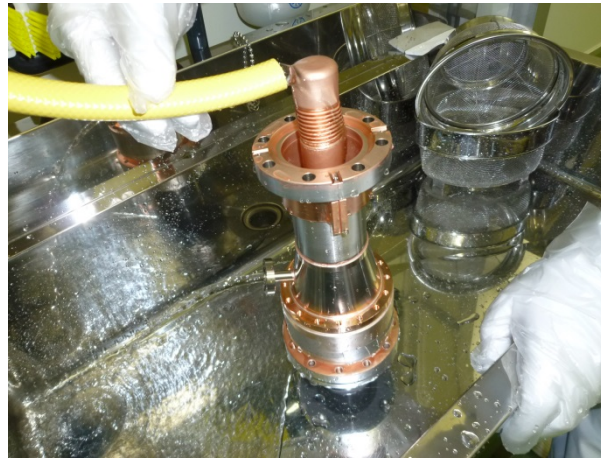
Low pressure water rinsing with ultra-pure water
