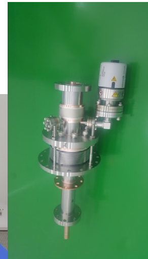
QWR Coupler for RAON (IBS/RISP) 81.25MHz
