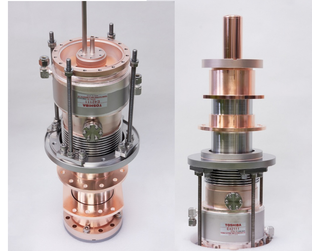
1.3 GHz cERL Injector Input Coupler (KEK)
