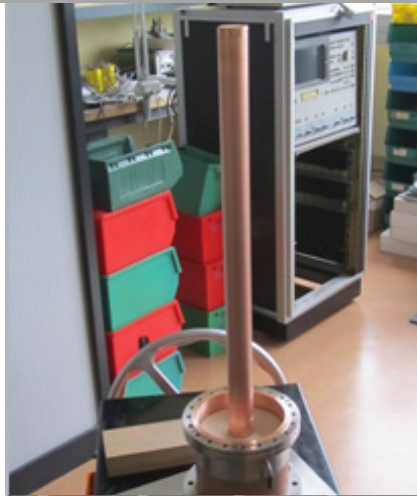
QWR Coupler for SPIRAL-2 (CEA-Saclay) 88MHz
