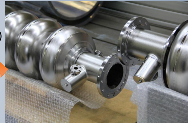
back-extruded Nb tubes for E-XFEL
