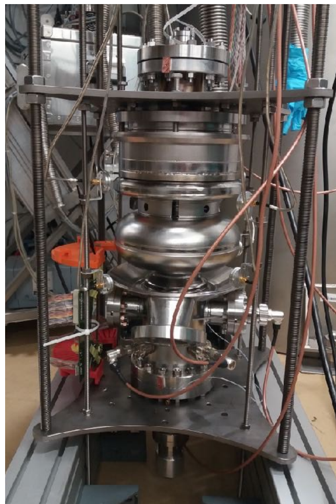
Gun I.1-cavity prepared for vertical testing
