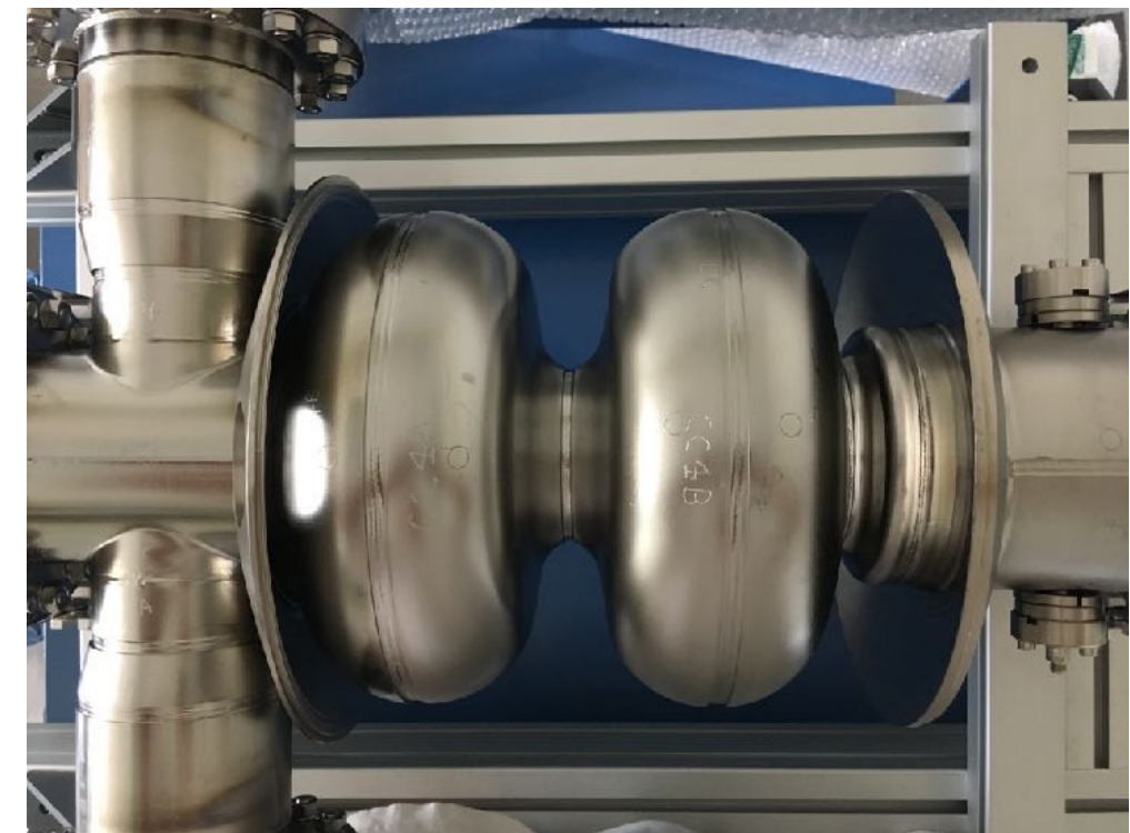
Cornell-style bERLinPro booster 1.3 GHz-2-cell without tank
