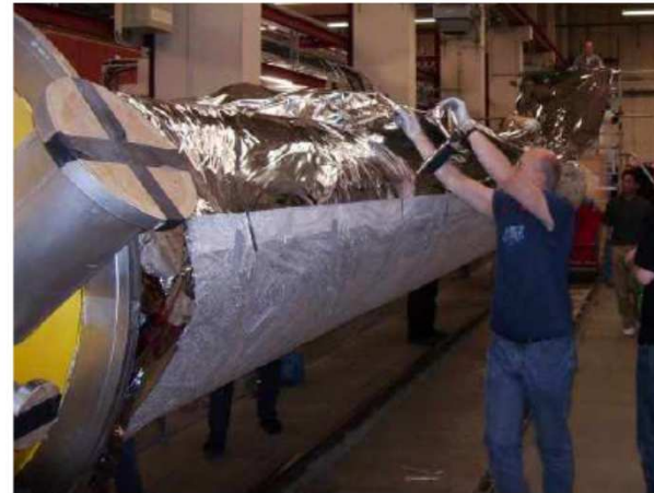
Figure 61: Two layers of super insulation on cold mass
