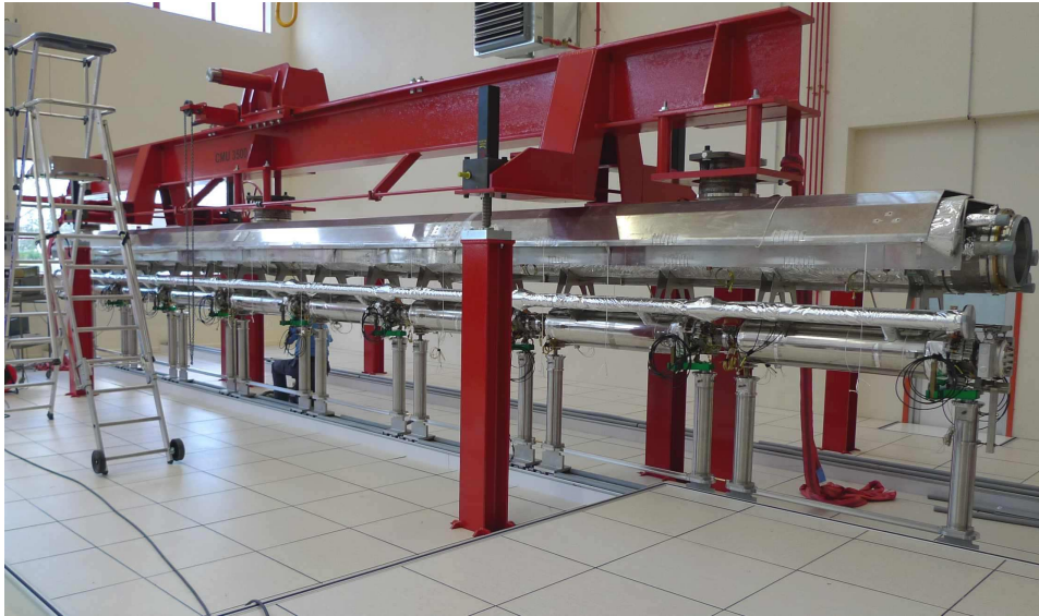
Cavity string is attached to cold mass
