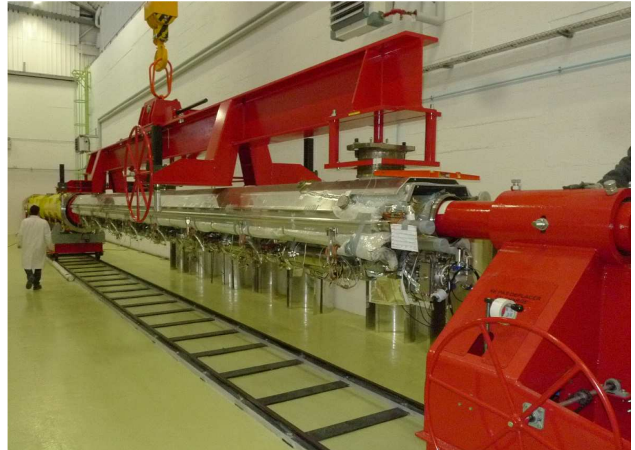
Tool to slide complete cold mass into vacuum vessel
