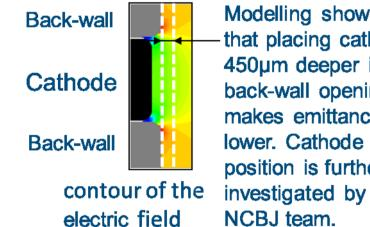
Modelling showed -that placing cathode 450µm deeper in the back-wall opening makes emittance lower. Cathode position is further NCBJ team.
