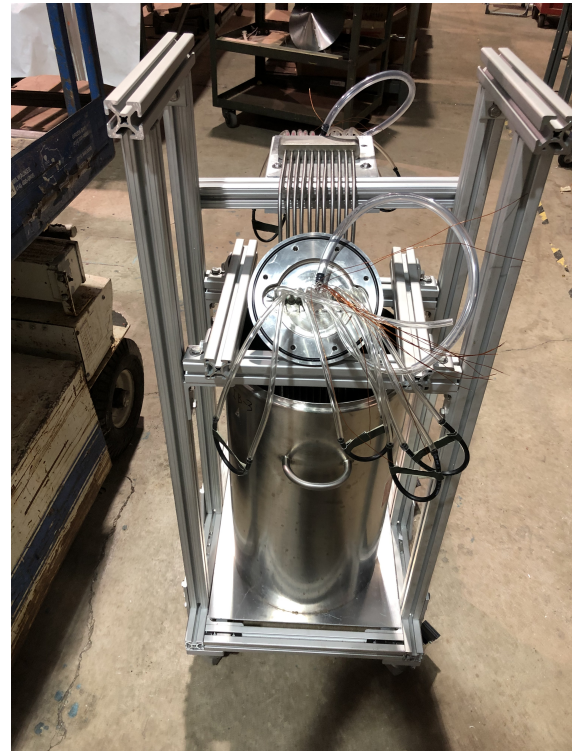
Figure 5: Current Leads Epoxy Filling Fixture.
