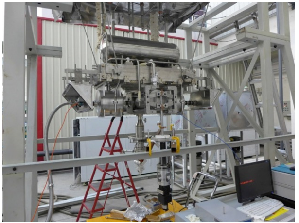
One cavity and two solenoids as prototype for assembly and tuning
