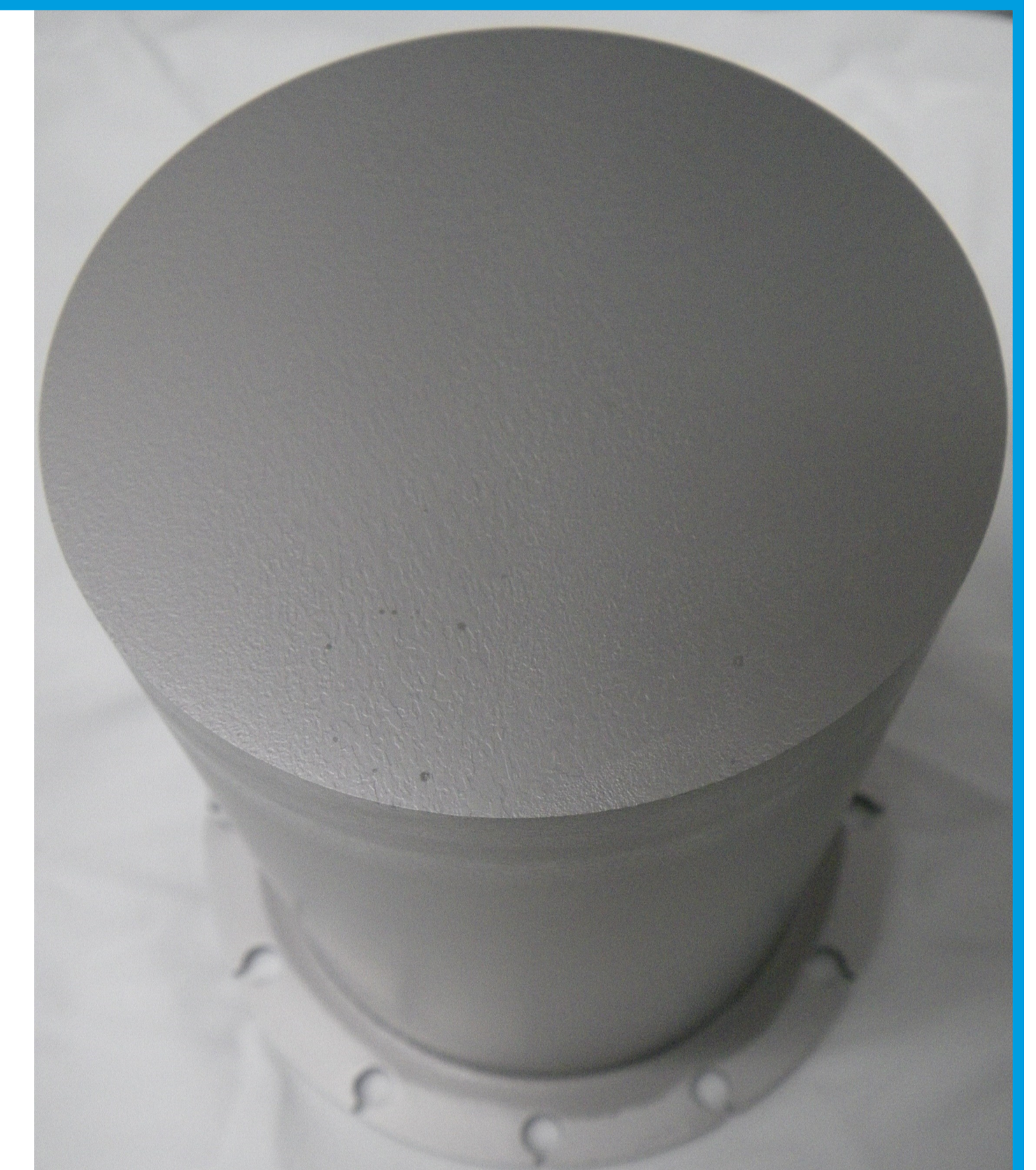
QPR sample after coating with Nb 3 Sn Coating procedure as for cavities [1]
