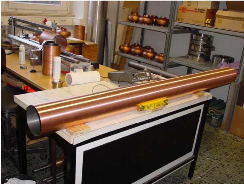
NbCu0.15%Zr tube, produced at Company NU-TECH Precision Metals (Canada)
