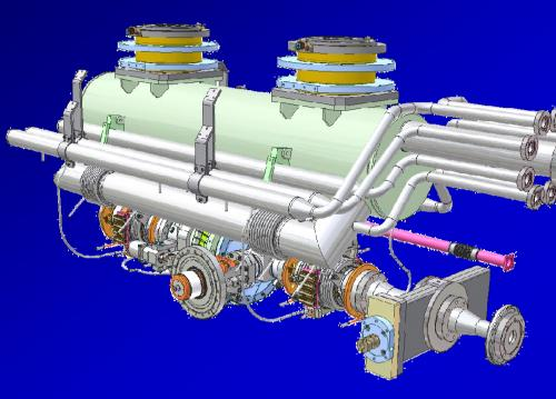
• Vacuum vessel will be used later as an ERL main linac cavity test cryomodule
