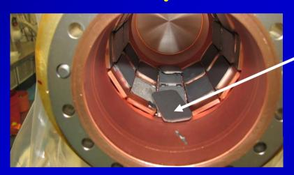
Two ferrite tiles cracked and dropped; found ferrite chips in the cavity beam pipe...
