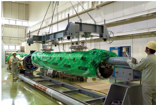
Remove cold mass of the downstream half cryomodule
