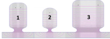
Figure 4: Electric field lines in the optimized buncher.
