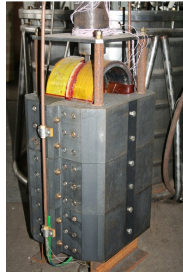
Figure 8: HTS dipole magnet on Bi2223 basis.
