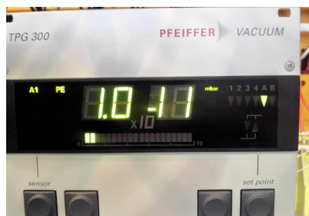
Figure 4: Vacuum in the cooler vacuum chamber.
