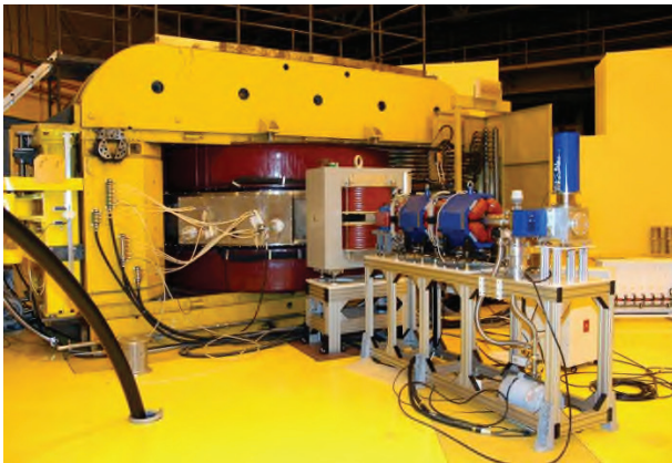
Figure 1: The external view of the C-80 cyclotron and beginning part of the transport line.
