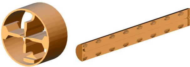
Figure 4: Optimized design of the SVRFQ cavity with elliptical coupling windows.
