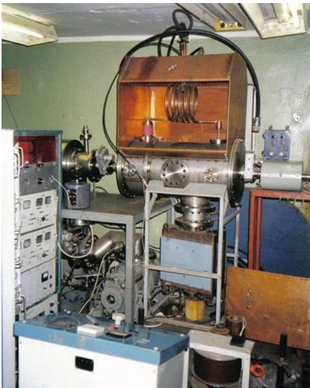
Figure 1: The 300 keV Implanter of single charged nitrogen ions.
