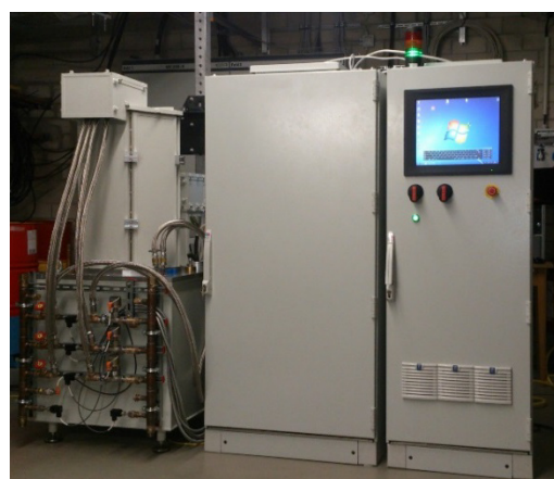
Figure 7: 130 kV modulator with pulse transformer.
