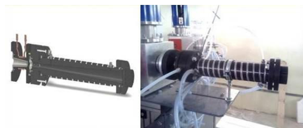
Figure 4: Target device for production of carbon-11 ( ^{11}\text{C} ) radionuclide.
