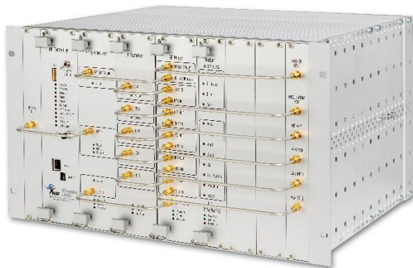
Figure 1: The new digital, low-level RF control system.
