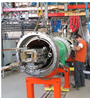
Figure 5: The dipole magnet inside the Booster cryostat.
