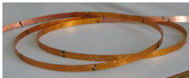
Figure 5: Insulated Rooble-type cable.
