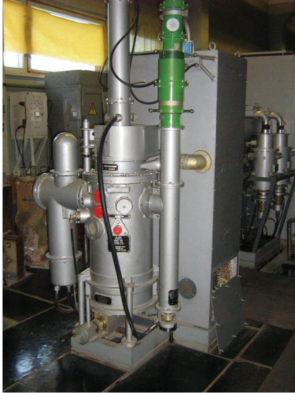
Figure 3: Intermediate power RF amplifier.
