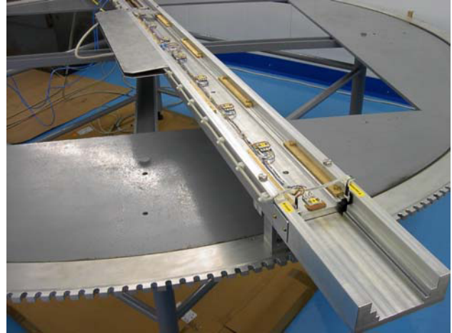
Figure 1: DC72 magnetometer with gear wheel.
