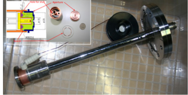
Figure 1: Pre-bunching triode cavity with longitudinal power coupling for a triode type thermionic RF gun.
