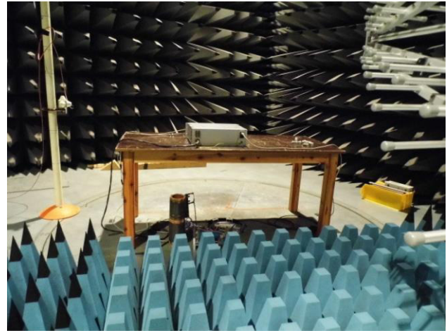
Figure 5: Test set-up for radiated susceptibility.
