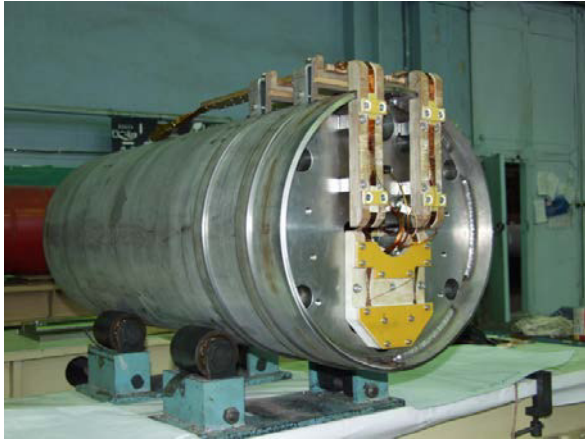
Figure 3: High field fast cycling dipole magnet.
