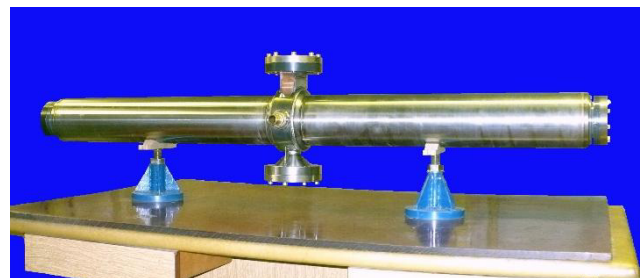
Figure 6: Accelerating structure with cooling jacket.
