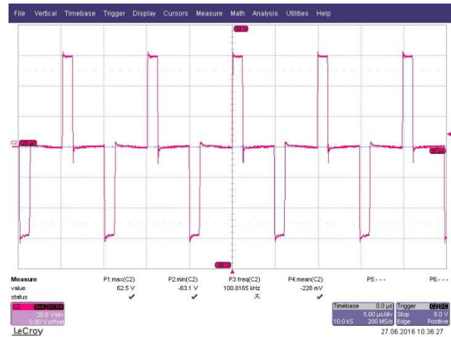
Figure 3: Oscillogram of H-Bridge Inverter output voltage.
