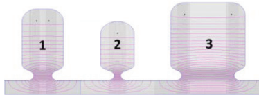
Figure 4: Electric field lines in the optimized buncher.
