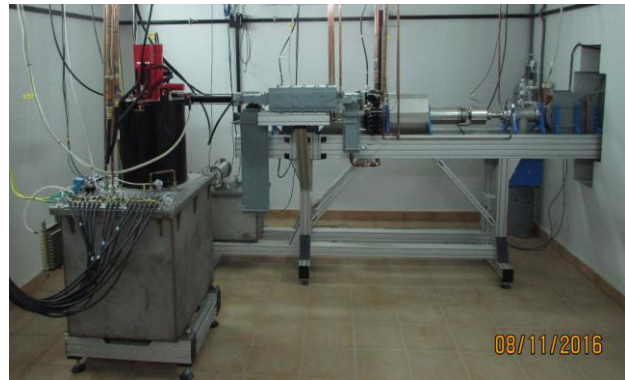
Figure 3: Photo of installed linac at ACCENTR Ltd. Company site, the beam scanner is clearly seen in the right side of the photo.
