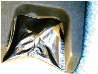
Figure 4: A damaged graphene foil.
