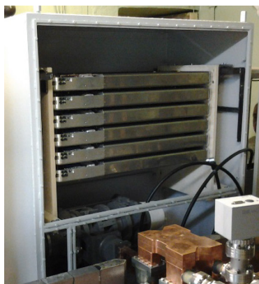
Figure 2: Direct switch solid-state 60 kV modulator.
