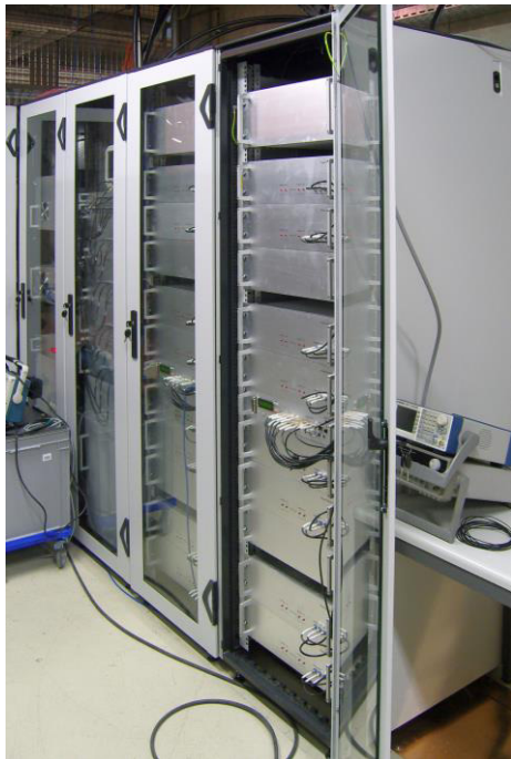
Figure 5: Four cabinets of RF generator. Nearest two racks are occupied by RFG20, next two contain DC power supply and final combiner.
