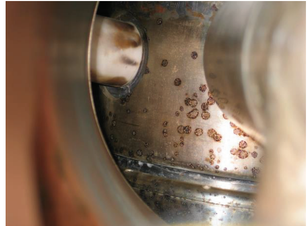
Figure 6: Traces of breakdowns in FPA plate-grid cavity.
