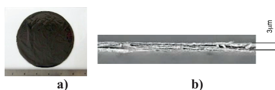
Figure 1: General view of graphene foils: a) fabricated foil; b) graphene cross section.
