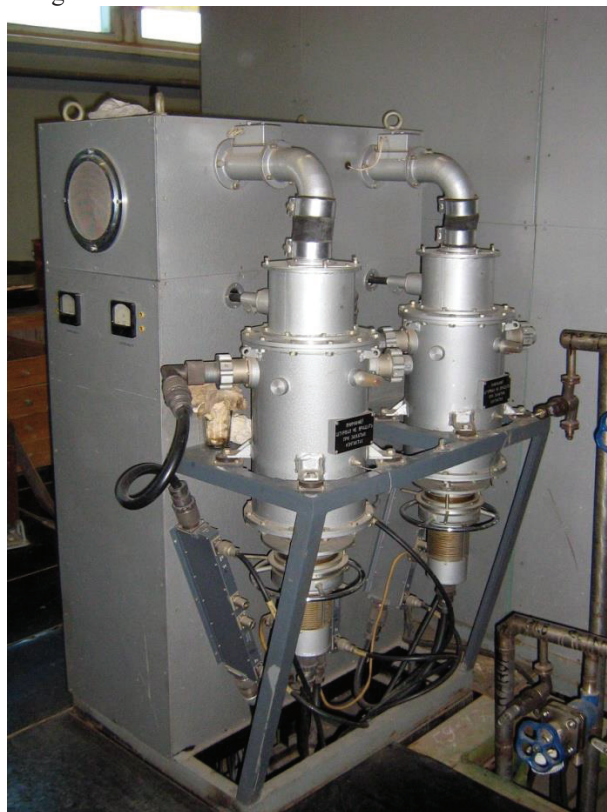
Figure 2: Two-stage RF amplifier.
