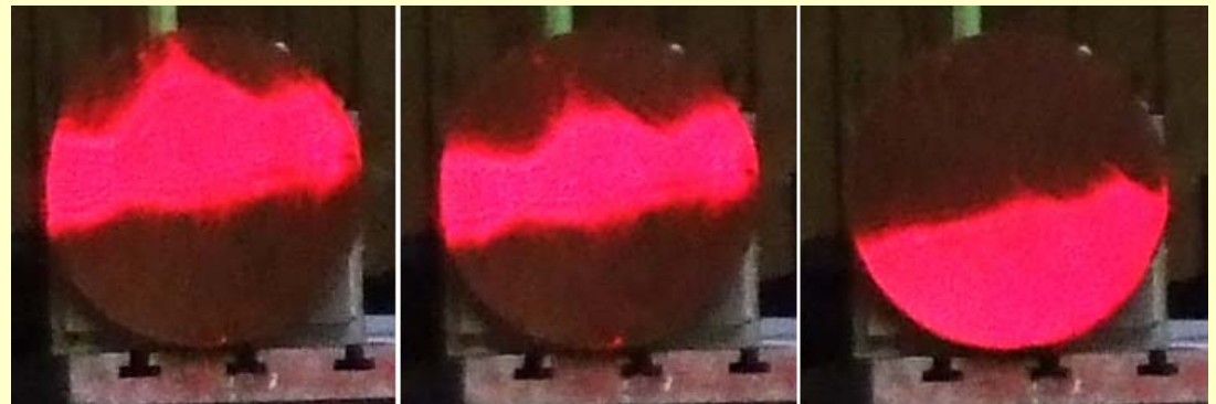
Image of a point radiation source transmitted by damaged mirror in optical telescope
