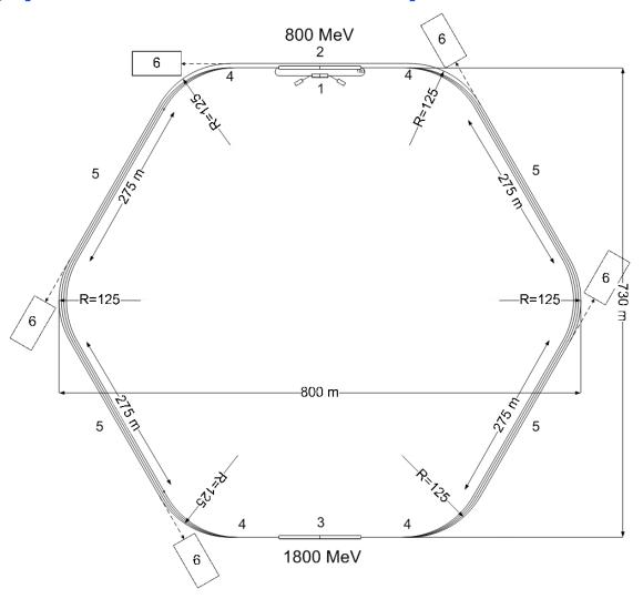
1 – injector, 2 – 1st linac, 3 – 2nd linac, 4 – spreders & recombiners, 5 – undulators, 6 – user stations
