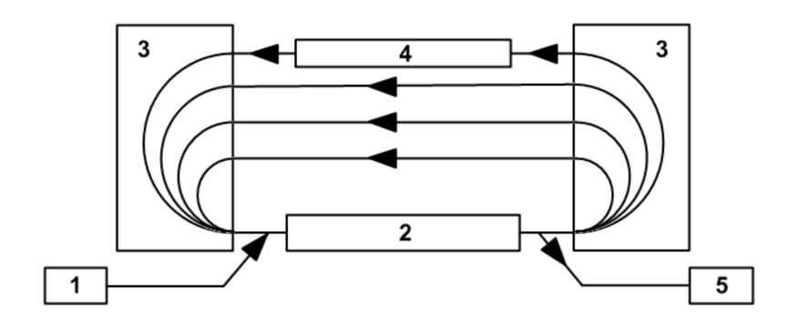
1 - injector, 2 - linac, 3 - bending magnets, 4 - undulator, 5 - dump
