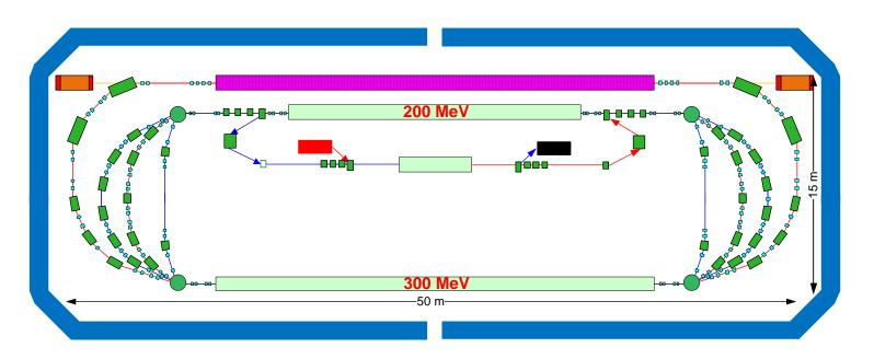
With 10-T superconducting magnet the 1-GeV ERL may be used to generate 20-fs periodic x-ray pulses, which are necessary for time-resolved experiments. Such experiments use femtoslicing technique at storage rings now. But, the number of useful photons at ERL will be thousands times more.
