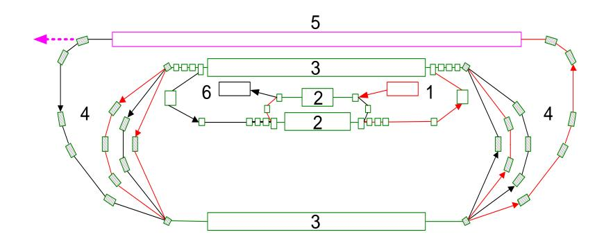
1 – injector, 2 – preliminary accelerating system, 3 – main accelerating RF structure, 4 – magnets, 5 – undulator, 6 – dump.
