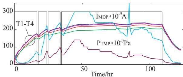
Figure 7: The baking out process. T1-T4 is temperatures of different sensors of the cavity in °C,  $I_{MDP}$  is the current of magnetic-discharge pump,  $P_{TMP}$  is the pressure measured at the turbo molecular pump connection.
