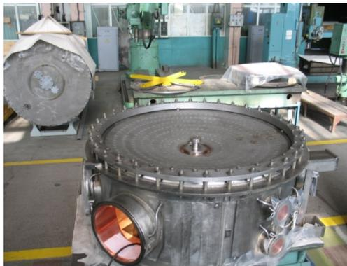
Figure 3: The left wall welding to the sidewall.
