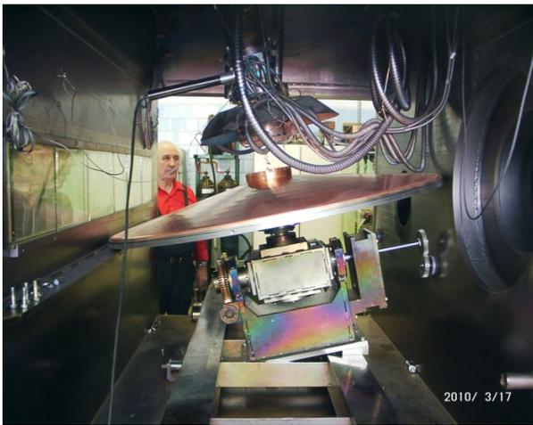
Figure 2: The left side wall with the cone nose installed into the vacuum chamber before the electron beam welding.
