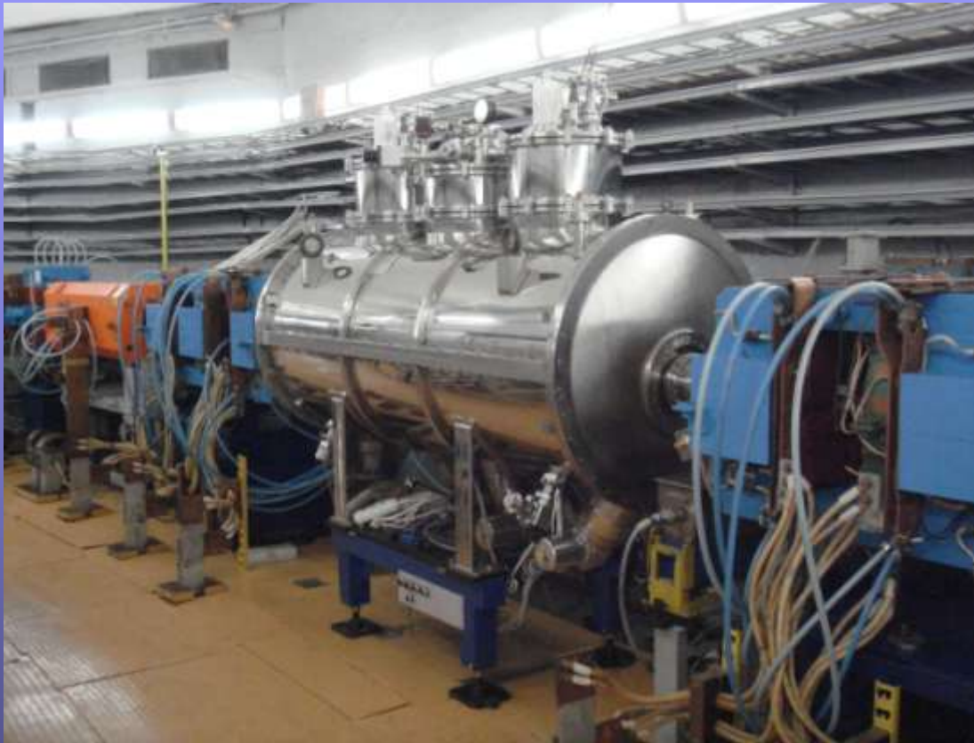
Superconducting wiggler in dispersion free straight section of SIBERIA-2.
