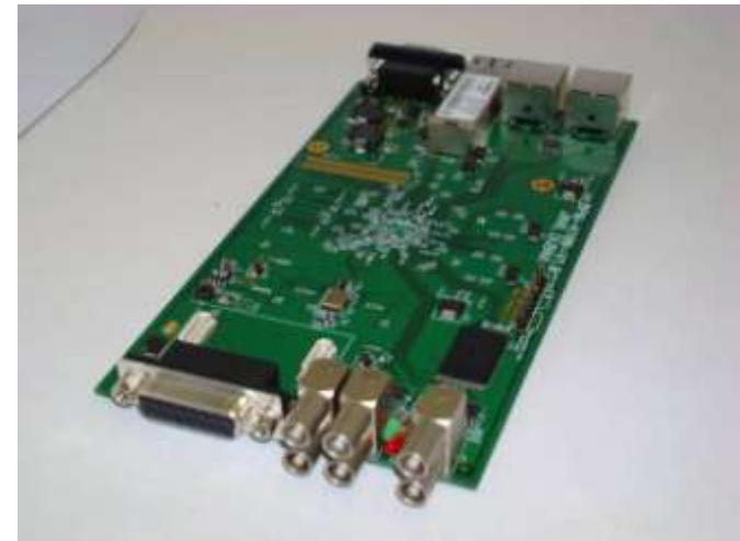
RuPAC2010 One of 30 chips (hi-tech) for automatic System for beam orbit measurement
