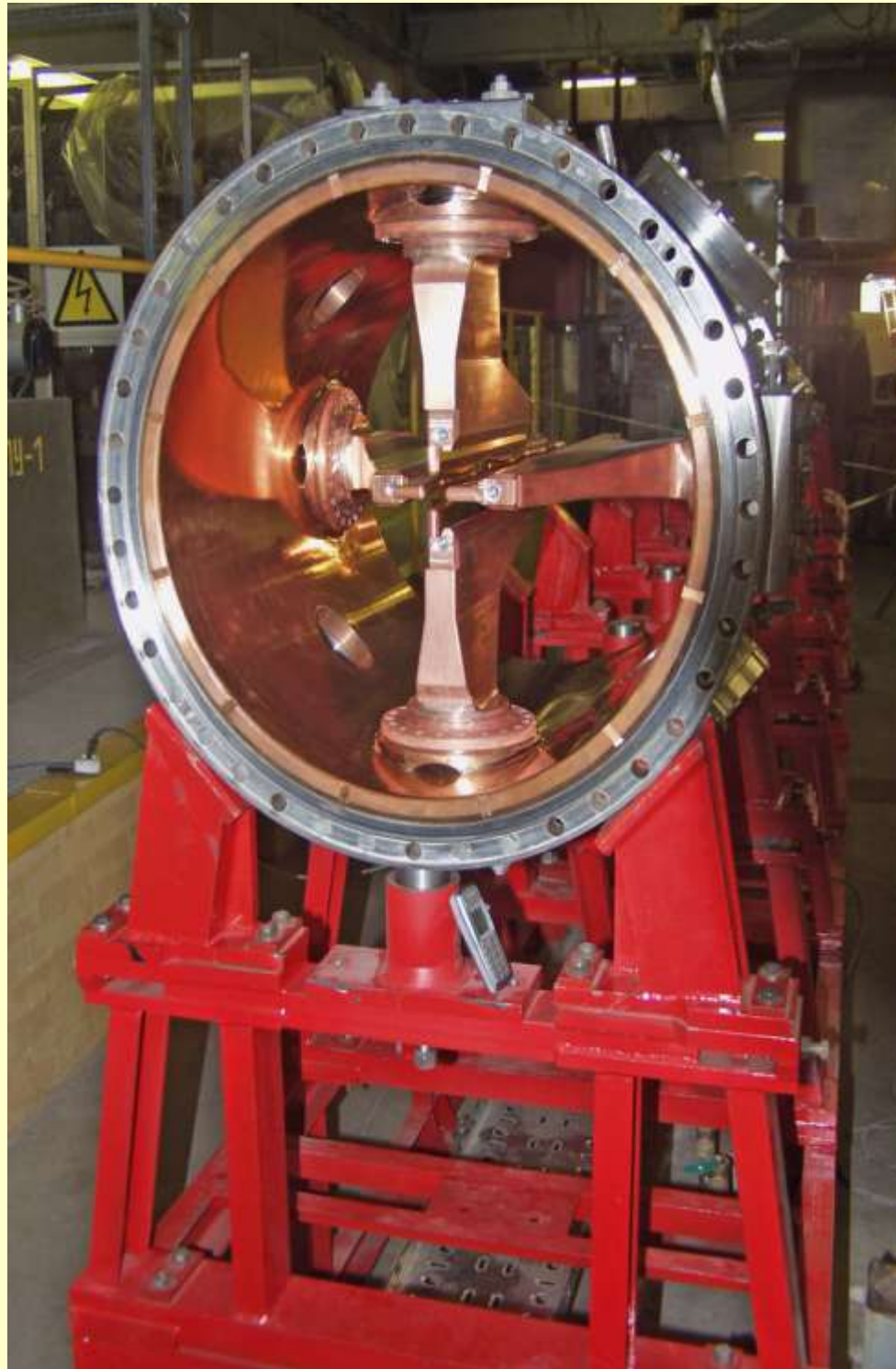
View of the RFQ with open outlet flange
