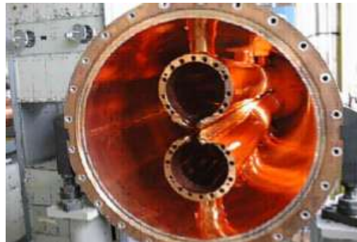
2H cavities of "Ural" RFQ (prototype)
