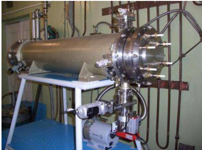
Assembled vacuum and cryogenic vessels of the KRION-6T
