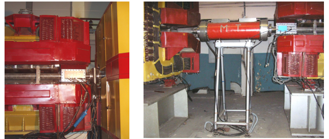
Figure 3: Pickup station (left). Electro-magnetic beam kicker followed by an auxiliary in-situ beam pickup (right).
