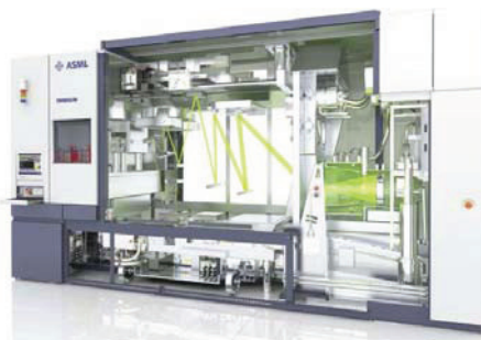
Figure 1: ASML TWINSCAN NXE industry platform for EUVL with LLP at radiation wavelength of 13.5 nm.
