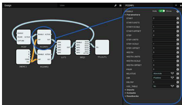
Figure 10: Web GUI interface showing an example application design with FBs.
