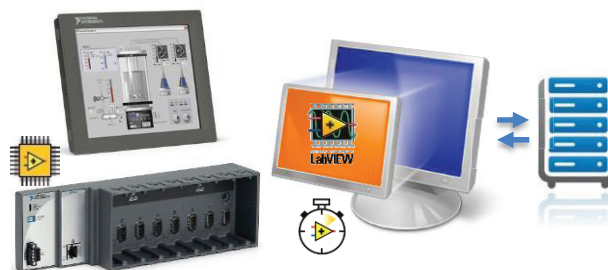
Figure 3: Schematic representation of the interface hardware, using NI cRIO with FPGA card, NI LabVIEW in virtual machine, data bank in central Storage System and NI Touch Panel for final user interface.
