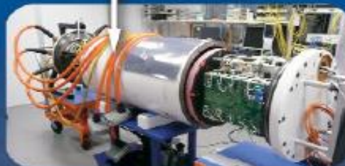
Low Voltage Power / Comms Assembly
