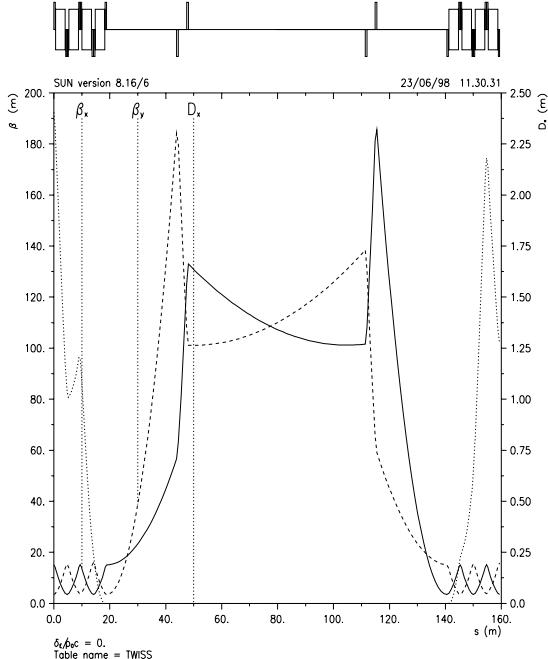
Figure 1: Initial design: The neutrino production region flanked by matching sections and dispersion-suppression cells
