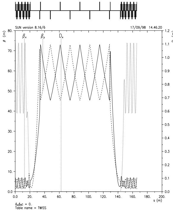
Figure 2: Later design: Lattice functions of the high-beta FODO cells for neutrino production flanked by matching sections, dispersion suppression cells, and three arc modules.
