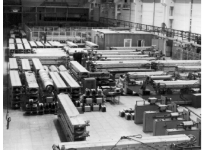
Figure 5: UNK-600 dipoles stored in the test facility building.
