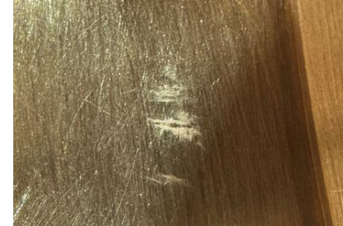
High temp CuCrZr normal incidence test thermal fatigue life at approximately 450°C
