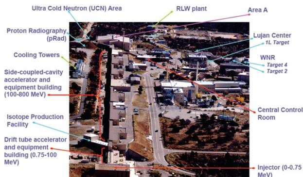
Figure 1: Layout of Los Alamos accelerator facility.
