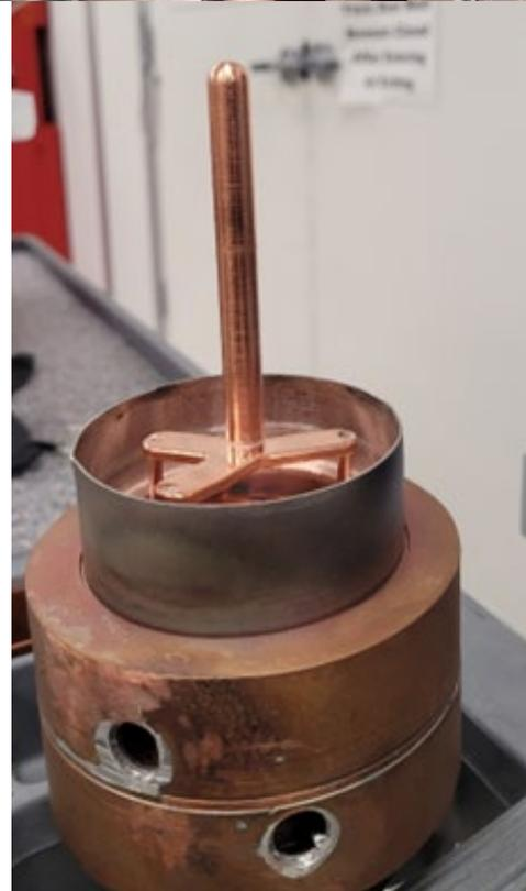
Figure 1: Photos show internal structure, ten cavities, straps and antenna attached to anode body. The new antenna design will have five legs.
