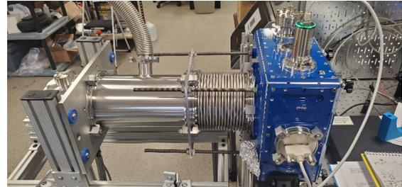
Figure 1: Vacuum envelope with the cryocooler and pumping port on the left and the (blue) instrumentation volume with feed-throughs on the right.
