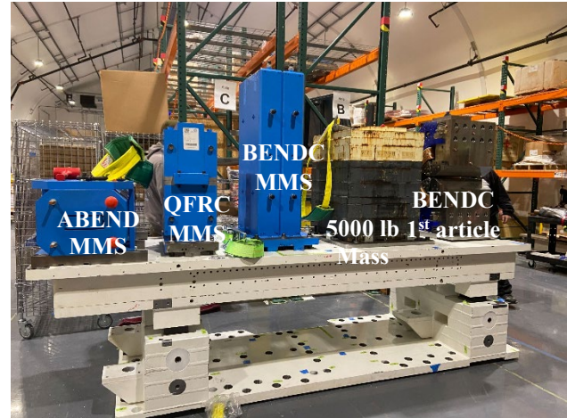
Figure 2: Storage ring prototype raft, configured for impact hammer testing.
