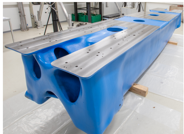
Figure 1: PETRA IV Demonstrator Girder.
