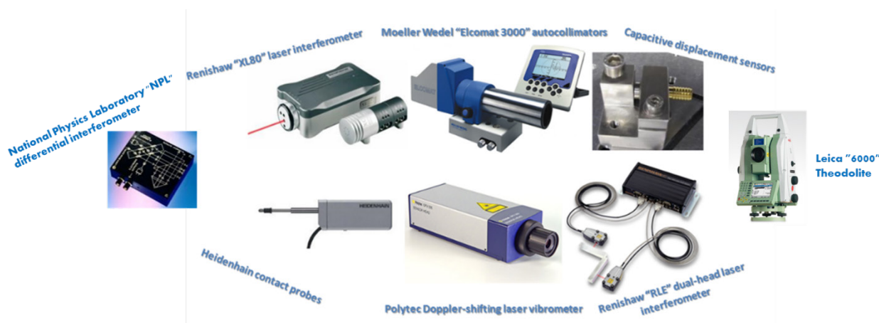
Figure 1: The Precision Metrology Laboratory provides an ultra-stable environment for micro- and nano-scale metrology characterisation of beamline motion stages using commercial and in-house-developed instrumentation.
