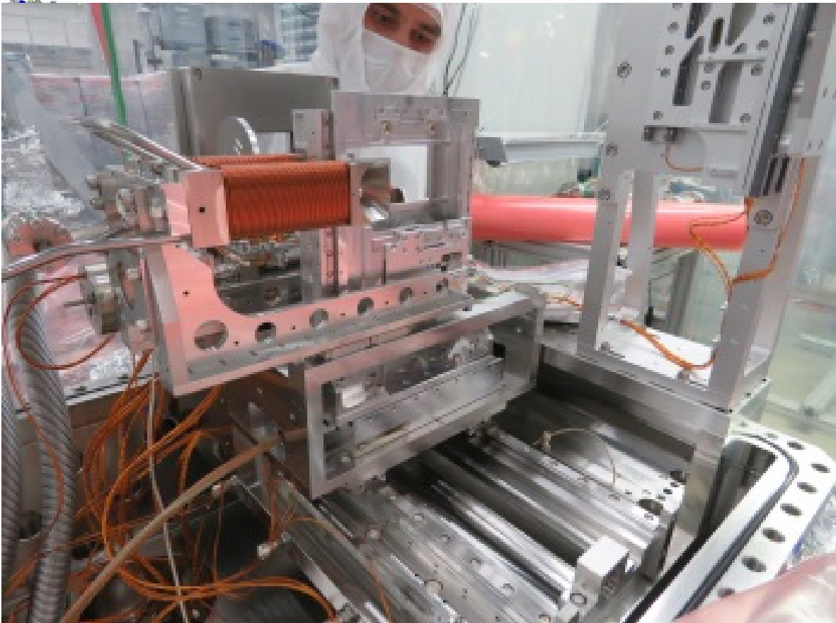
10 Hz XY-scanner with twin coil magnet and transferable sample frame with load-lock
