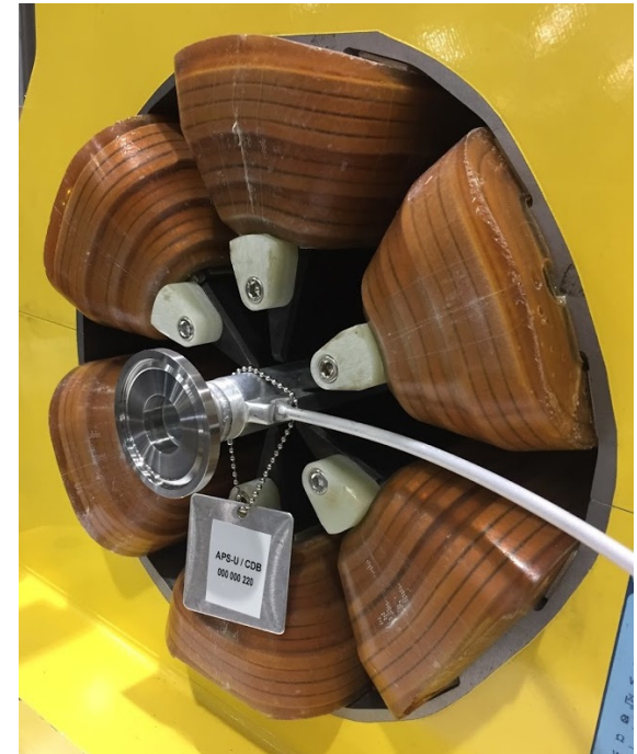
Existing APS storage ring chamber compared to new 22 mm ID APS-U style chamber
