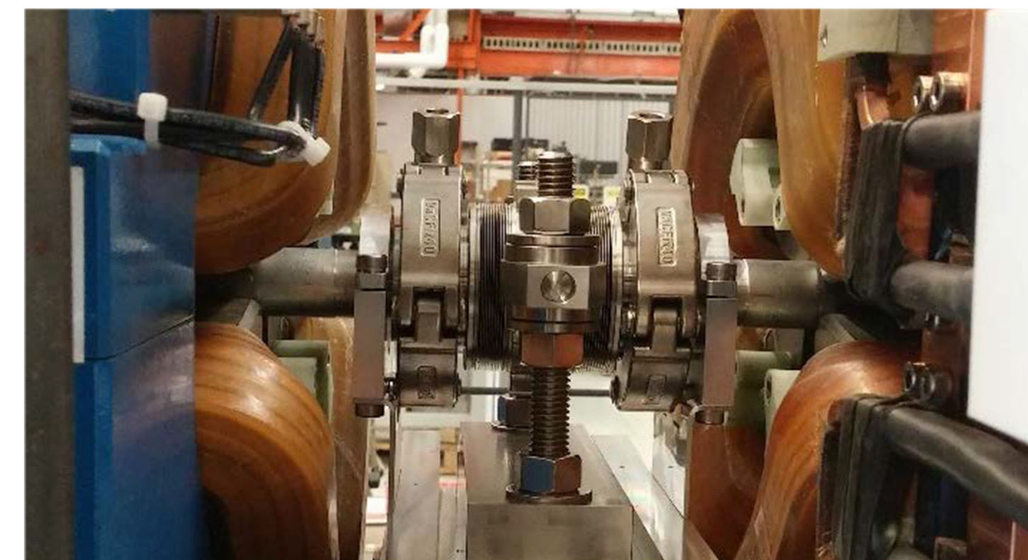
Mockup of compact BPM between two quadrupole magnets
