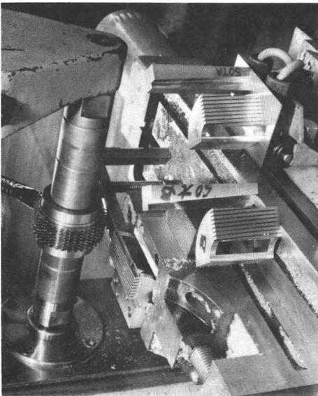
Fig.7 Cutting of the parallel grooves by a milling machine.
