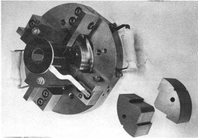
Fig.11 Assembling of the cores and coil on a jig.
