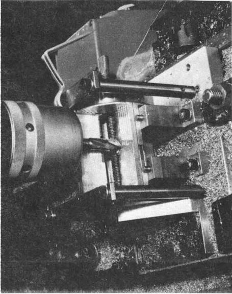
Fig.9 Final machining of assembled coil.
