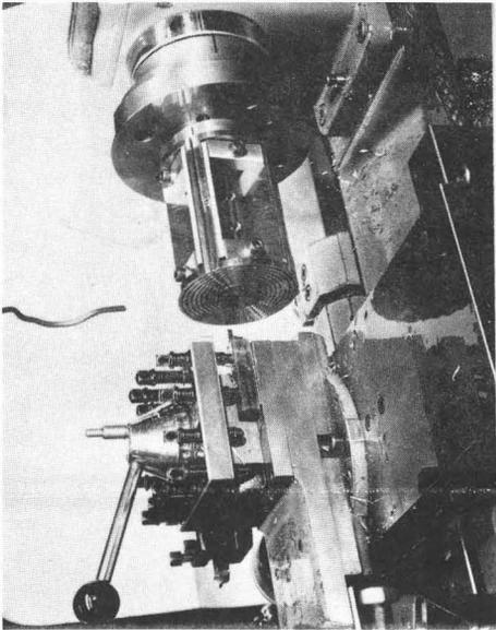
Fig.8 Cutting of the azimuthal grooves by a lathe.
