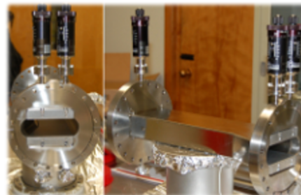
Figure 1: Dipole chamber with adjustable shielding gap.
