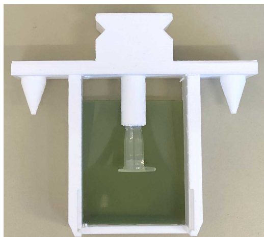
Figure 3: Picture of the 3D printed holder with a PCR tube and a radiochromic film. Note that the ZFE are kept in the cap of the tube for the irradiation.
