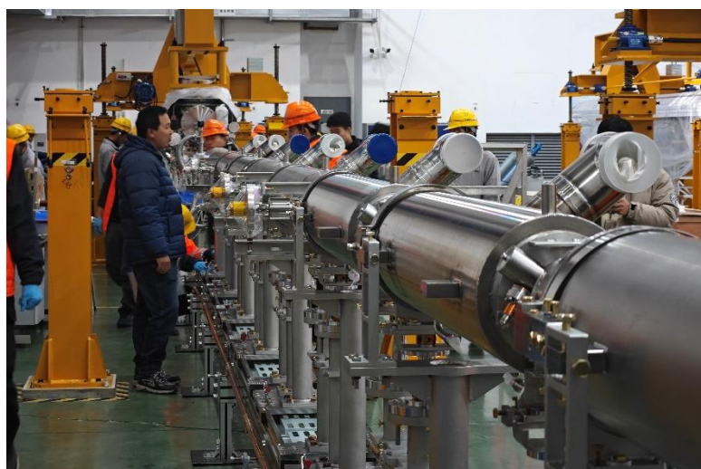
i8CM for Injector (8 midT cav.)
