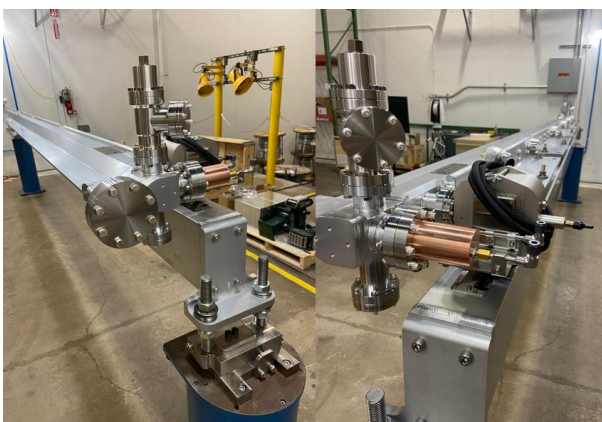
Figure 8: The new ID vacuum chamber undergoing pre-alignment in preparation for storage ring installation. Left: Thin-nose view. Right: Rear-side (outboard) view. The downstream photon absorber is seen at the near end in both views.
