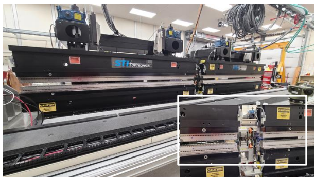
Figure 4: Photograph of two 2.5-cm-period HPMUs with phase shifter and corrector in the middle (insert) measured on the 6-m bench in the magnet measurement laboratory.
