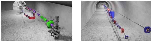
Figure 3: Renders of the 3D model of the cooler and hadron beamlines in the RHIC tunnel. Left: the injector, low energy merge, linac entrance, and return line featuring a Bates bending system; right: the amplifier and hadron beamline.
