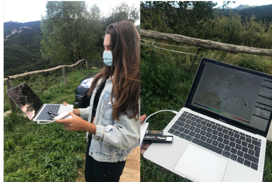
Xènia Turró, from INS Vilafant measuring natural radiation in Tapís (Maçanet de Cabrenys). She identified the various particles in the environment coming from different sources and compared the measured radiation dose with the recommendations from the International Commission on Radiological Protection.
