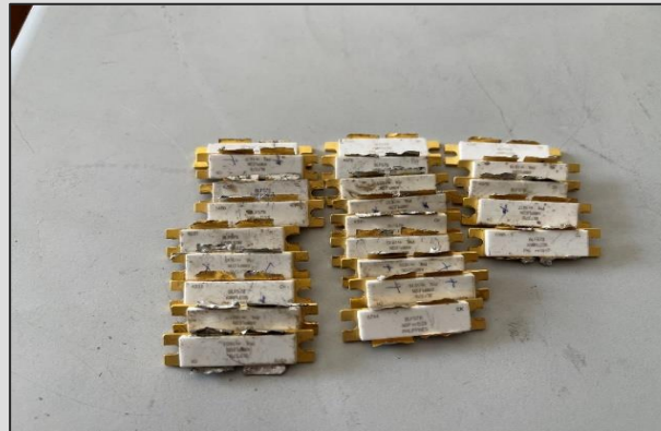
Harvest of broken transistors BLF578
