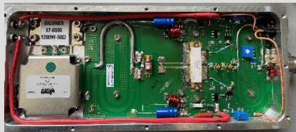
Inside view of 550 W RF module
