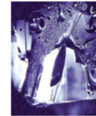
Photograph of the liquid lithium film charge stripper in the Facility for Rare Isotope Beams. Selected for a Synopsis in Physics [Kanemura et al. Phys. Rev. Lett. 128 , 212301 (2022)]
