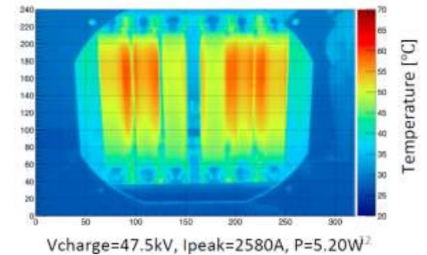
\* Inj Kickers need to manage beam induced current. Newly designed system demonstrated the surface temperature of their resistors below their threshold 150 °C for high voltage impulses (eq. 1.3 MW op.)
