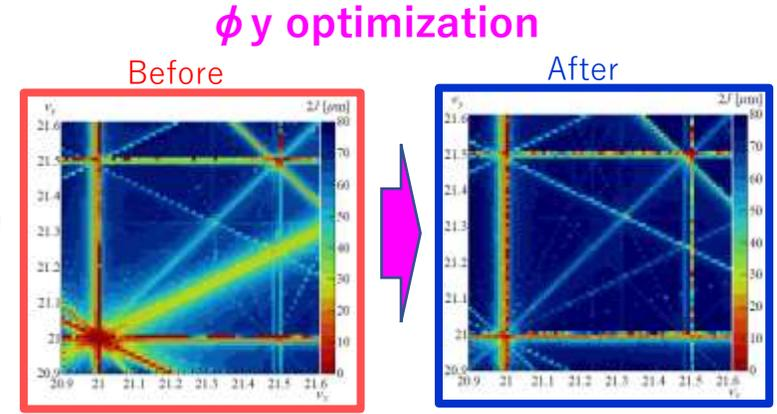
Dynamic aperture survey of single particle (SAD)
