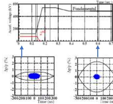
Simulated longitudinal motion for 1.16 s cycle (including beam loading & long-SC)
