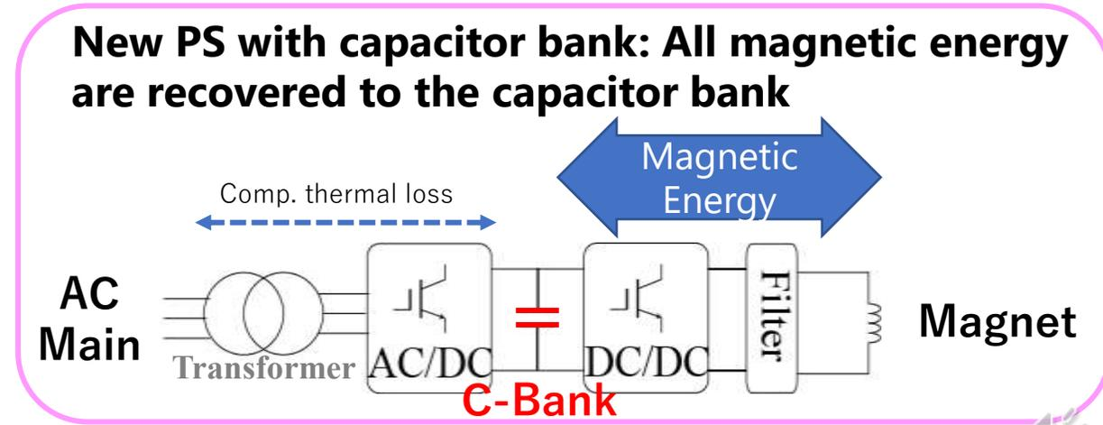
\* One PS drives several magnets connected in series. These several magnets are collectively called "a Family"
