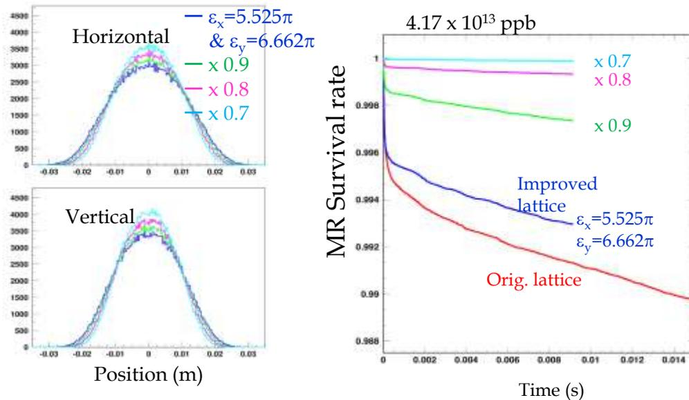
In JFY2020, RCS optimization has been done for MR beam for 1.3 MW eq. protons per bunch. Beam emittance was reduced with the new tune setting in RCS.
