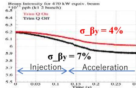
Long. bunch oscillation of 480 kW beam
