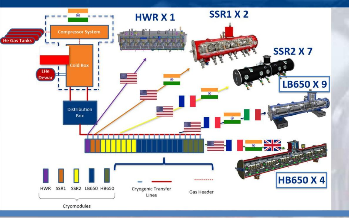
Fermilab is upgrading its existing accelerator complex to support a world leading neutrino program and future high intensity frontier particle physics experiments. At PIP-II core is the design and construction of a Continuous Wave (CW) superconducting radio frequency (SRF) linear accelerator that would accelerate an average beam current of 2 mA up to 800 MeV. PIP-II beam acceleration occurs mainly in SRF CW linac that will employ five different types of superconducting cavities.
