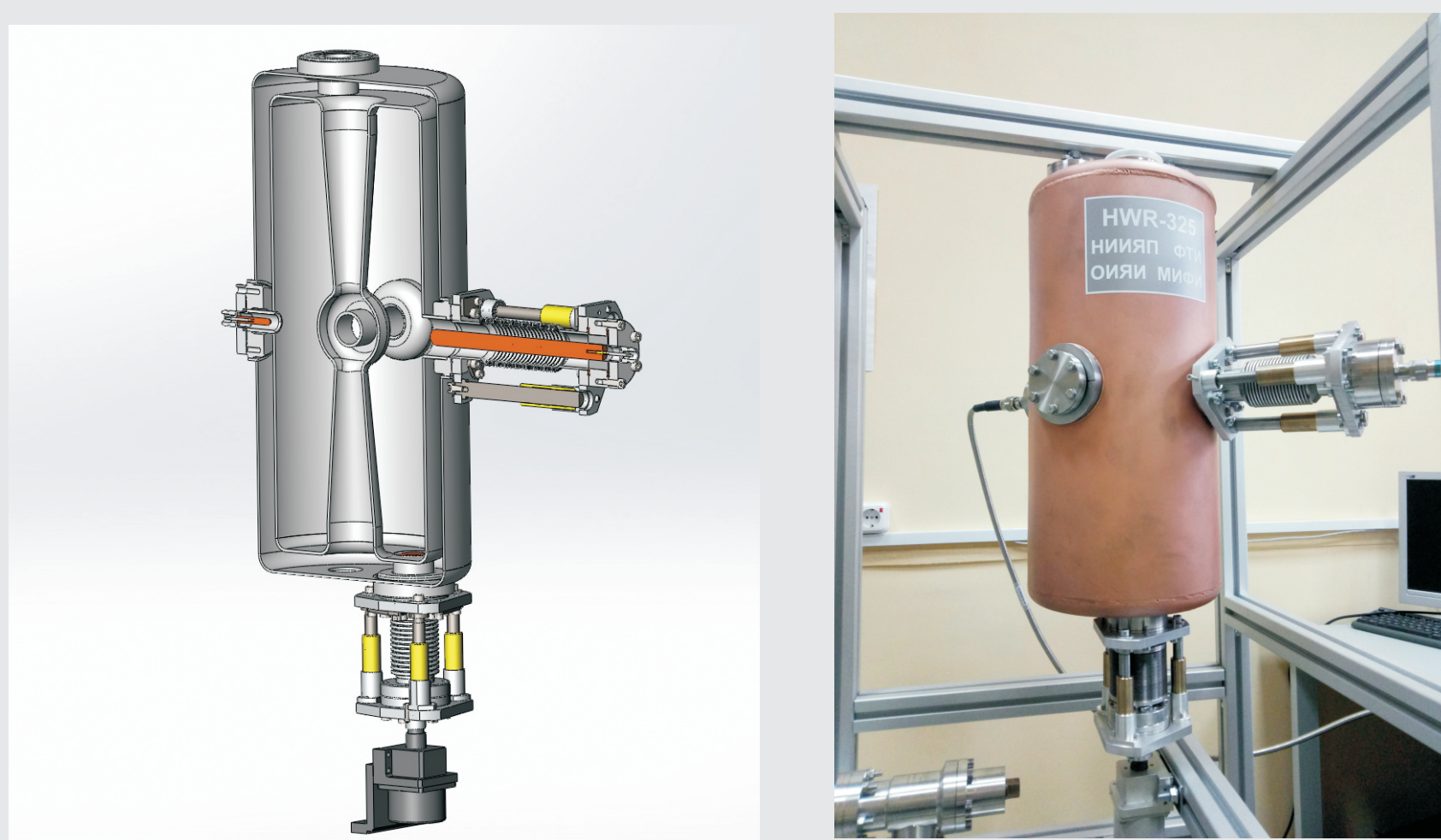
Figure 1. 325 MHz HWR cavity mode (left), fabricated copper prototype (right).
