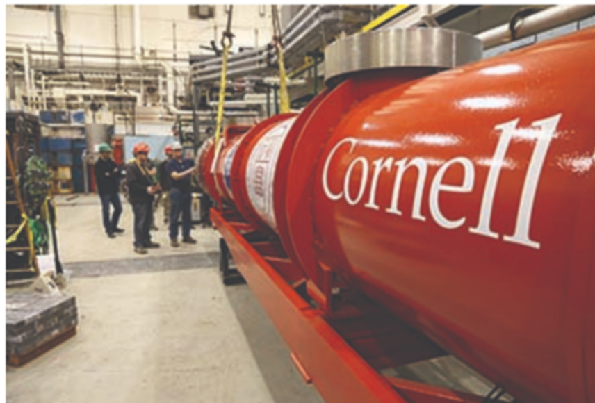
The main linac cryomodule
