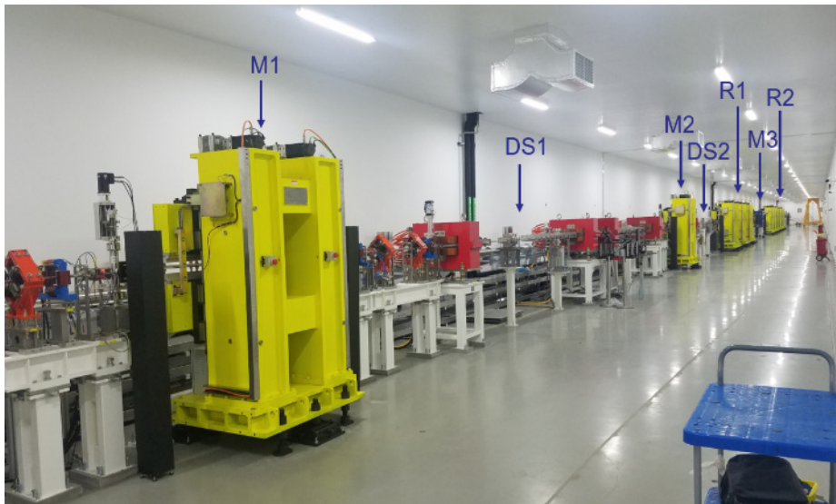
Layout for the echo-30 experiment at SXFEL
