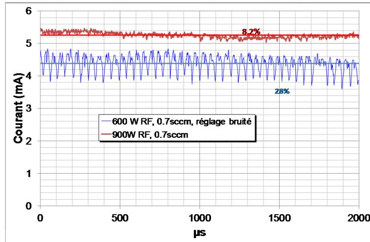
Ability to extract **11 mA CW** from source => up to **6 mA** proton beam at the RFQ entrance
