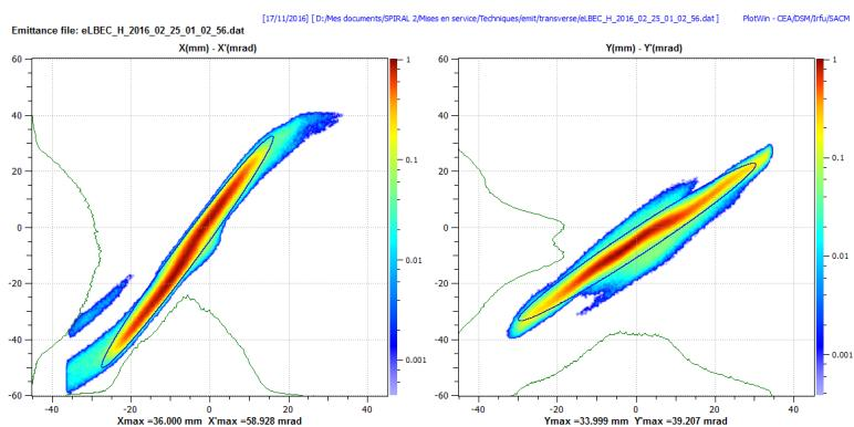
5.2mA H<sup>+</sup>, 0.2  $\pi \text{ mm mrd rms norm.}$
