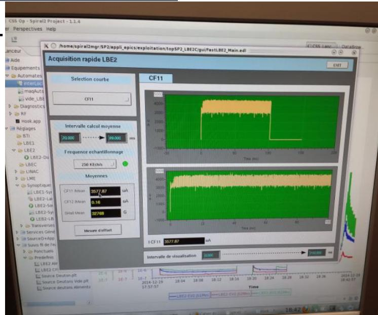
Ability to extract **11 mA CW** from source => up to **6 mA** proton beam at the RFQ entrance
