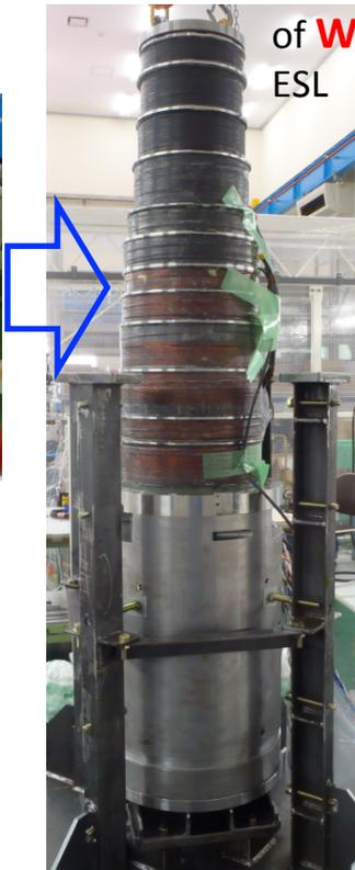
Assembling the radiation shield of W alloy on ESL
