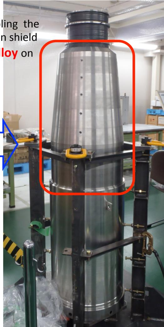
Covering the cold mass with the helium vessel and welding the vessels
