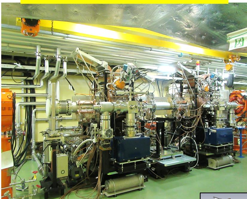
\* High-power RF conditioning was completed at a test stand for each cavity.
