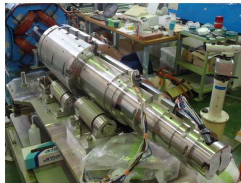
Combination of the cold mass and the ESL solenoid
